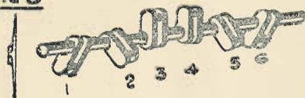
Crankshaft for 6 Cylinder Vertical engine or 6x2 Cylinder "Vee" engine as in 140. H.P. R.A.F.
