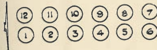
System of numbering cylinders in 6x2 cylinder "Vee" engine
